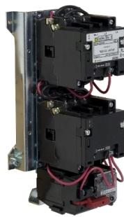
NEMA starter, Type S, reversing, vertical, Size 1, 27A, 10HP at 575VAC, up to 100kA SCCR, 3 phase, 3 pole, Motor Logic SSOLR, 120VAC coil, open [TAA]
