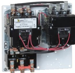
NEMA starter, Type S, reversing, horizontal, Size 3, 90A, 50HP at 575VAC, 5kA SSCR, 3 phase, 3 pole, melting alloy overload, 120VAC coil, open [TAA]
