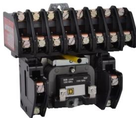
Contactor, Type L, multipole lighting, electrically held, 30A, 10 pole, 600V, 110/120VAC 50/60Hz coil, open style [TAA]
