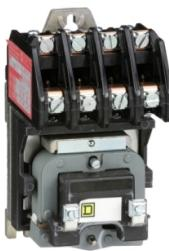
Contactor, Type L, multipole lighting, electrically held, 30A, 4 pole, 600V, 277VAC 60Hz coil, open style [TAA]
