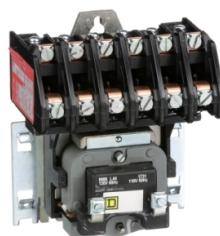
Contactor, Type L, multipole lighting, electrically held, 30A, 6 pole, 600V, 110/120VAC 50/60Hz coil, open style [TAA]
