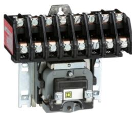
Contactor, Type L, multipole lighting, electrically held, 30A, 8 pole, 600V, 277VAC 60Hz coil, open style [TAA]
