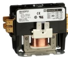
Contactor, Definite Purpose, 30A, 1 pole, 24/24VAC 50/60Hz coil, open
