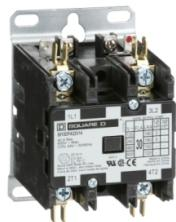
Contactor, Definite Purpose, 30A, 2 pole, 5HP at 230VAC, 1 phase, 24VAC coil at 50/60Hz, open
