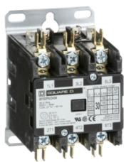
Contactor, Definite Purpose, 30A, 3 pole, 20HP at 575VAC, 3 phase, 277VAC 60Hz coil, open
