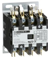
Contactor, Definite Purpose, 30A, 4 pole, 20HP at 575VAC, 3 phase, 208/240VAC 60Hz 220VAC 50Hz coil, open
