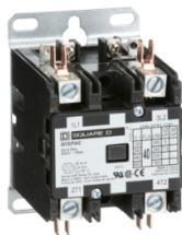
Contactor, Definite Purpose, 40A, 2 pole, 7.5HP at 230VAC, 1 phase, 24/24VAC 50/60Hz coil, open
