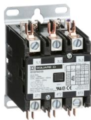
Contactor, Definite Purpose, 40A, 3 pole, 25HP at 575VAC, 3 phase, 208/240VAC 60Hz 220VAC 50Hz coil, open
