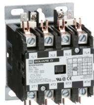
Contactor, Definite Purpose, 40A, 4 pole, 25HP at 575VAC, 3 phase, 110/120VAC 50/60Hz coil, open
