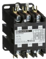
Contactor, Definite Purpose, 50A, 3 pole, 30HP at 575VAC, 3 phase, 24/24VAC 50/60Hz coil, open
