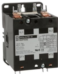
Contactor, Definite Purpose, 90A, 2 pole, 20HP at 230VAC, 1 phase, 110/120VAC 50/60Hz coil, open
