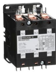
Contactor, Definite Purpose, 90A, 3 pole, 50HP at 575VAC, 3 phase, 208/240VAC 60Hz 220VAC 50Hz coil, open
