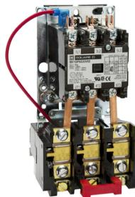
NEMA starter, Definite Purpose, 25A, 20HP at 600VAC, 3 phase, 3 pole, melting alloy, 480VAC coil, open
