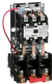
NEMA starter, Definite Purpose, 40A, 25HP at 600VAC, 3 phase, 3 pole, melting alloy overload, 24VAC coil, open
