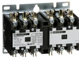
Reversing Hoist Contactor, 30A, 3 pole, 110/120VAC 50/60Hz coil, open style
