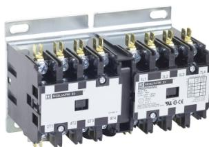
Reversing Hoist Contactor, 30A, 4 pole, 110/120VAC 50/60Hz coil, open style
