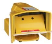
Foot Switch, Harmony 9002AW, industrial, oversized pedal and safety and side shields, SPDT contact, NEMA 4, 13, two stage, 5A at 600V AC
