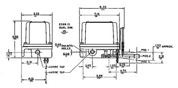
The alternating of two pumps takes place at position 2. Position 1 is reached only when one pump is unable to control the liquid level.
