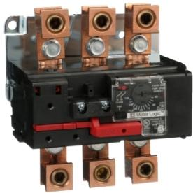
Overload Relay, Motor Logic, solid state overload relay, NEMA Size 4, 3 pole, 45A to 135A, 600VAC, separate mount
