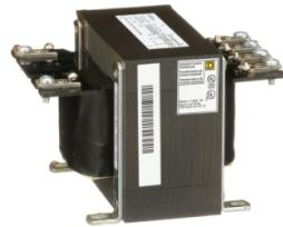
Transformer, EO, industrial control, 300VA, 1 phase, 240x480V primary, 120V secondary, 80C rise
