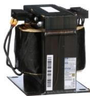
Transformer, Type T, industrial control, 1000VA, 1 phase, 240/480/600V primary, 120V secondary, 115C rise
