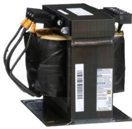
Transformer, Type T, industrial control, 1000VA, 1 phase, 240/416/480/600V primary, 99/120/130V secondary, 115C rise
