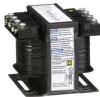
Transformer, Type T, industrial control, 100VA, 1 phase, 120V primary, 12/24V secondary, 55C rise
