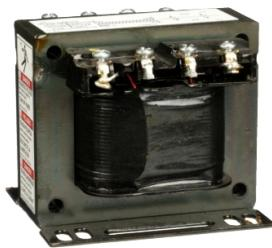
Transformer, Type T, industrial control, 100VA, 1 phase, 208V primary, 24V secondary, 55C rise
