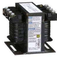
Transformer, Type T, industrial control, 100VA, 1 phase, 240x480V primary, 120V secondary, 55C rise
