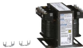
Transformer, Type T, industrial control, 100VA, 1 phase, 120x240V primary, 24V secondary, 55C rise
