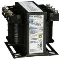
Transformer, Type T, industrial control, 100VA, 1 phase, 240x480V primary, 120/240V secondary, 55C rise
