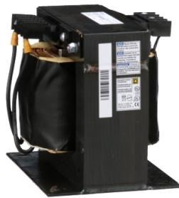
Transformer, Type T, industrial control, 1500VA, 1 phase, 380/400/415V primary, 115/230V secondary, 115C rise
