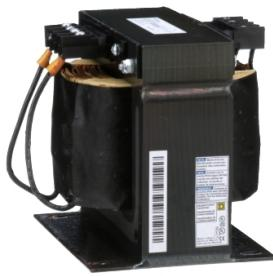
Transformer, Type T, industrial control, 1500VA, 1 phase, 208V primary, 120V secondary, 115C rise
