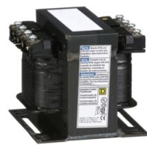
Transformer, Type T, industrial control, 150VA, 1 phase, 120x240V primary, 24V secondary, 55C rise
