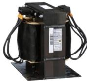
Transformer, Type T, industrial control, 2000VA, 1 phase, 208/230/460V primary, 115V secondary, 115C rise
