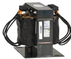
Transformer, Type T, industrial control, 2000VA, 1 phase, 240/416/480/600V primary, 99/120/130V secondary, 115C rise
