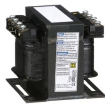
Transformer, Type T, industrial control, 200VA, 1 phase, 240x480V primary, 25/120V secondary, 80C rise
