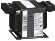
Transformer, Type T, industrial control, 250VA, 1 phase, 208V primary, 24V secondary, 80C rise
