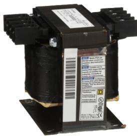
Transformer, Type T, industrial control, 250VA, 1 phase, 208/230/460V primary, 115V secondary, 80C rise
