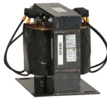
Transformer, Type T, industrial control, 3000VA, 1 phase, 480V primary, 240V secondary, 115C rise
