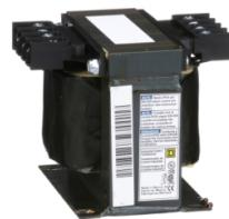
Transformer, Type T, industrial control, 300VA, 1 phase, 120x240V primary, 24V secondary, 80C rise
