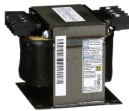
Transformer, Type T, industrial control, 500VA, 1 phase, 120V primary, 12/24V secondary, 115C rise
