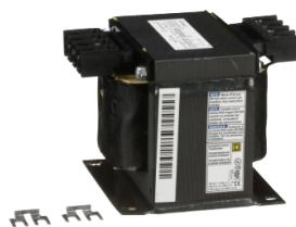
Transformer, Type T, industrial control, 500VA, 1 phase, 550/575/600V primary, 120/240V secondary, 115C rise
