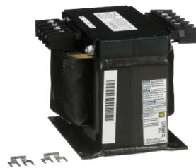
Transformer, Type T, industrial control, 500VA, 1 phase, 240/416/480/600V primary, 99/120/130V secondary, 115C rise
