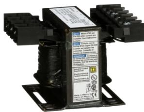
Transformer, Type T, industrial control, 50VA, 1 phase, 208/240/277/380/480V primary, 24V secondary, 55C rise
