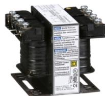
Transformer, Type T, industrial control, 50VA, 1 phase, 240x480V primary, 120V secondary, 55C rise
