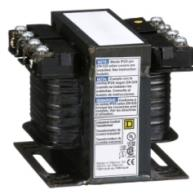
Transformer, Type T, industrial control, 50VA, 1 phase, 240/480/600V primary, 120V secondary, 55C rise
