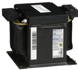
Transformer, Type T, industrial control, 750VA, 1 phase, 208/230/460V primary, 115V secondary, 115C rise
