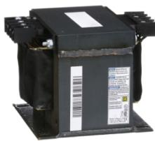
Transformer, Type T, industrial control, 750VA, 1 phase, 240/480/600V primary, 120V secondary, 115C rise
