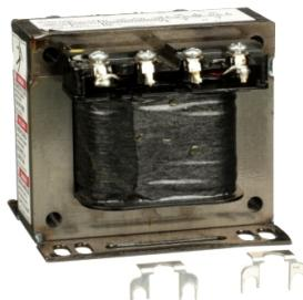
Transformer, Type T, industrial control, 75VA, 1 phase, 240x480V primary, 24V secondary, 55C rise
